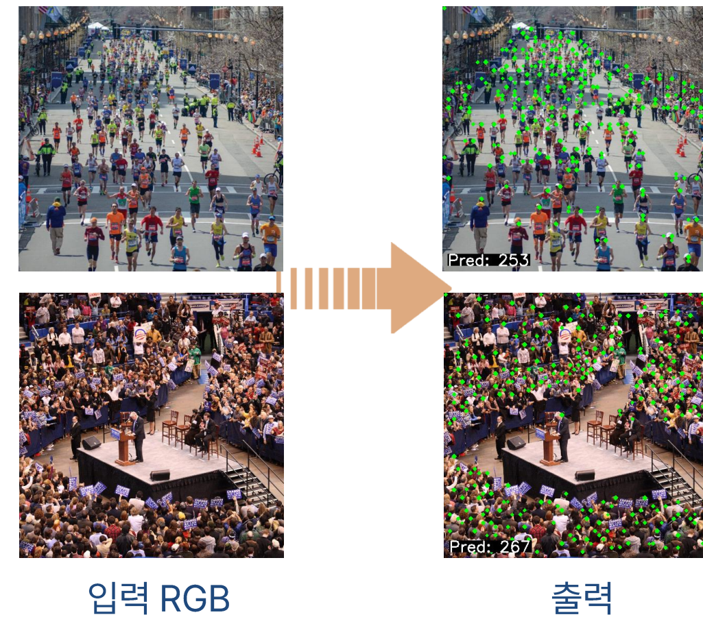
Figure 2. The output of our model when given an RGB image input. Green dots are marked on the part where the human head is recognized.
